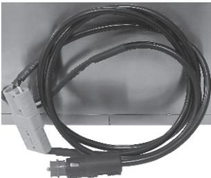
Three plug configurations - 12V, 50 Amp connector and Merit
