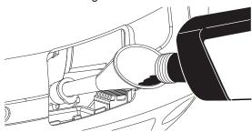
NOTICE Pause to permit oil to settle. DO NOT overfill.
