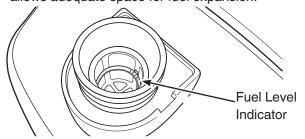
9. Install fuel cap and let any spilled fuel evaporate before starting engine.
