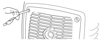
2. Remove screw that attaches spark arrester screen to muffler. Remove spark arrester screen.
