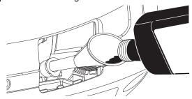
5. Replace and tighten oil fill cap.
