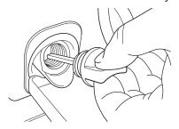
Using an oil funnel, slowly pour contents of oil bottle into oil fill opening. Checking oil level frequently, fill to point of overflowing.
