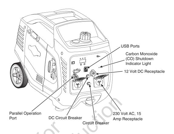
12 Volt DC Receptacle — Use this receptacle to supply power for 12 Volt DC accessories that are rated 60 watts (5 Amp) or less. This receptacle is protected by a push to reset circuit breaker.
