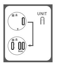
The scale contains both unit systems: metric (kg,g) and imperial (lb,oz). Press the UNIT button to convert between the two systems. (You'll see the UNIT button at the bottom of the product, as shown left.)
